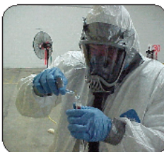
A STERIS Defense & Industrial technician collects biological indicators which were used to validate the efficacy of the decontamination process.
